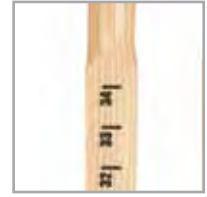
Inch marks to be used for depth measurements
