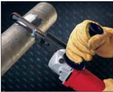
Strap polishing using contact arm 48-08-0290.
