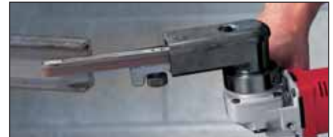
Grind and deburr ends of metal stock.
