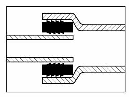
The donut is designed to provide several points of seal in order to accommodate possible irregularities in the pipe surfaces. If one seal-point is disturbed, the others will maintain the seal.
